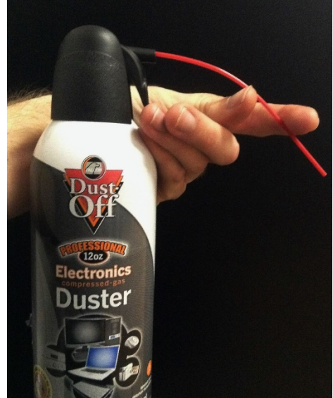
Figure 5: Correct vertical orientation of air-duster bottle. Air is blown at an angle by bending the attached plastic nozzle.
