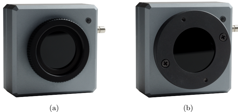
Figure 1: (a) C-Mount ND filter attached to a WinCamD-LCM4. The ND C-Mount filters are set at a 3^\circ in their case to prevent reflection and interference effects. (b) MagND filter attached to a WinCamD-LCM4. The MagND filters are set at a 2^\circ in their respective cases to prevent reflection and interference effects.
