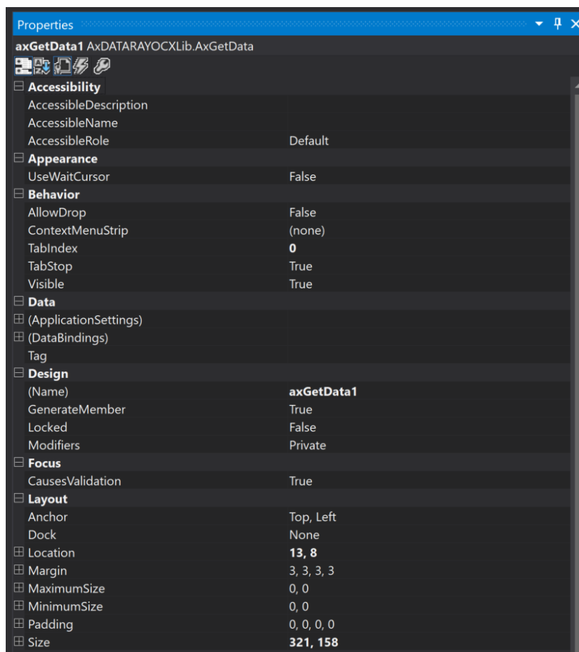
Figure 8: By default when you add the GetData Control it will create a member called axGetData1 . This object contains the method StartDriver() that needs to be called to initialize the camera. You can change the name of this variable by highlighting the GetData Control editing the properties and changing the name.
